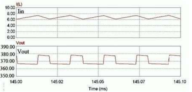
Fig.3: Input current and output voltage waveform of conventional bi-directional DC-DC converter during step up mode.
